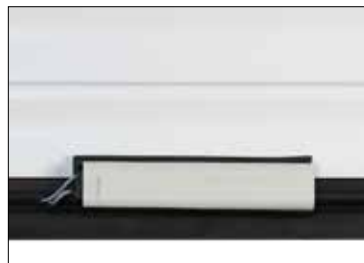
Wireless optical sensor (batteries required)
